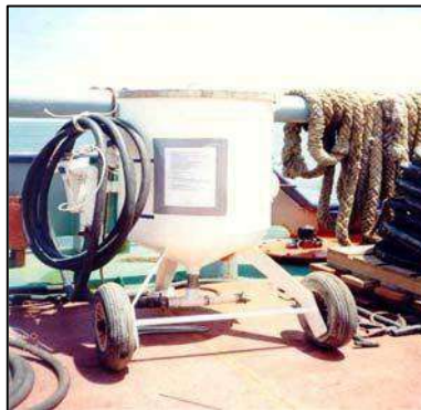
GRIT BLASTING UNIT
