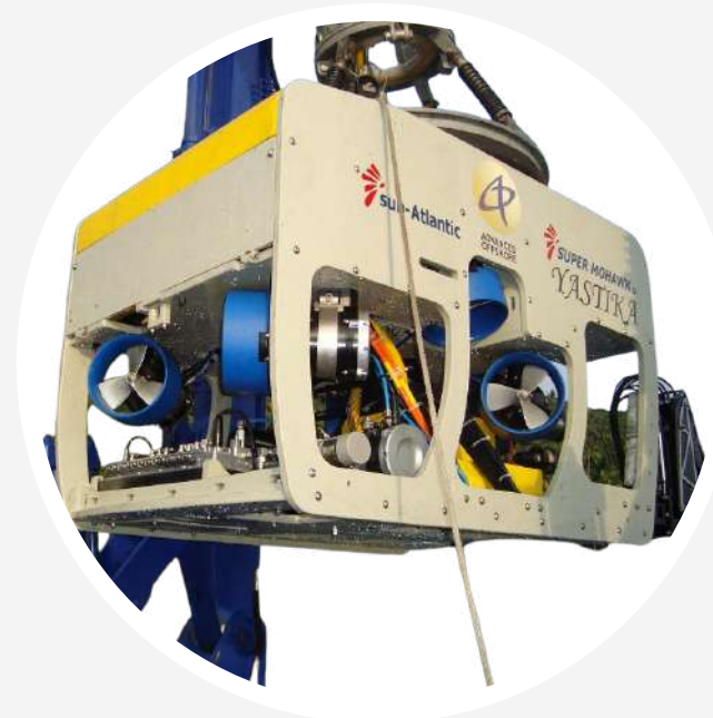
Inspection Class ROV Supermohawk
